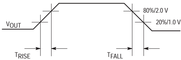
Figure 3. Rise and Fall Times
