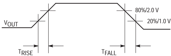
Figure 3. WAVEFORMS: Rise and Fall Times
